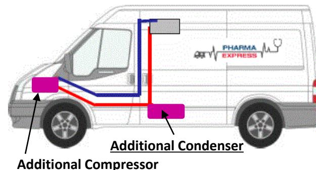
The Pharma Power Plus system **is complete independent** from the vehicle original HVAC system with a additional Pharma compressor and undermount condenser.
